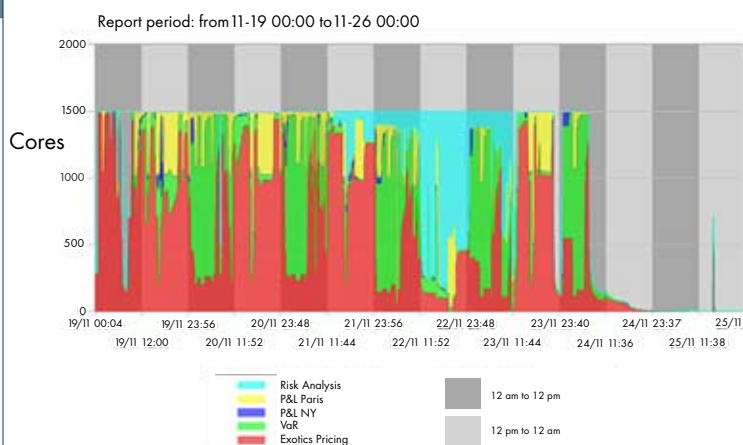
Figure 1. This diagram illustrates how matching applications with complementary usage patterns can maximize utilization of cores in a grid. In addition to matching applications that run at night to those that peak during the day, the bank also co-locates applications from different geographical locations to take advantage of the time differences.
